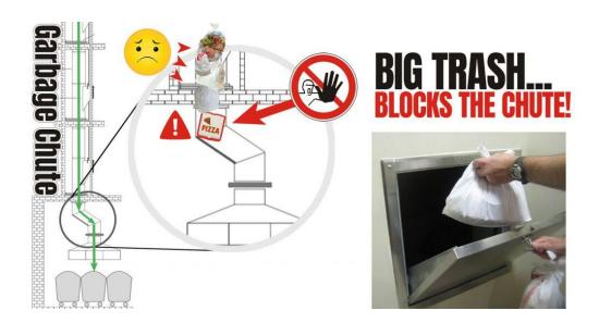
The garbage chute has an angle at the bottom—if you throw boxes, oversized trash bags, or long objects that obstruct the elbow, the entire chute gets jammed. If you have trash that is larger than a standard grocery bag in width or height, do not force it down the chute; take it down to the dumpster at the ground floor (Northeast Front).
